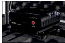
The CLF W-Bridge is a complete plug and play wireless DMX kit which includes a transmitter/receiver, receiver, antennas and CLF Tourcase. The W-Bridge uses the Wireless Solution® protocol to ensure a reliable wireless transmission of one DMX universe (512 channels).
